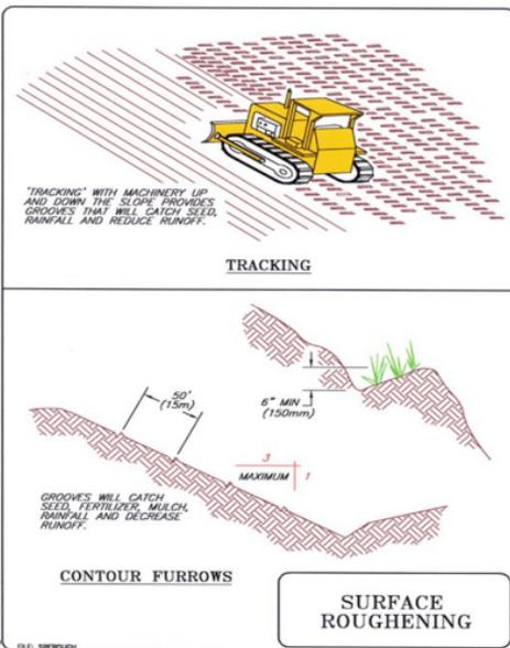
Roughening is best used on 3:1 slopes that do not require mowing. On steeper slopes, 2:1 or greater, a stair-step pattern (terracing) should be formed. Adding organic material such as straw mulch prior to tracking will further reduce erosion by up to an additional 80%.
