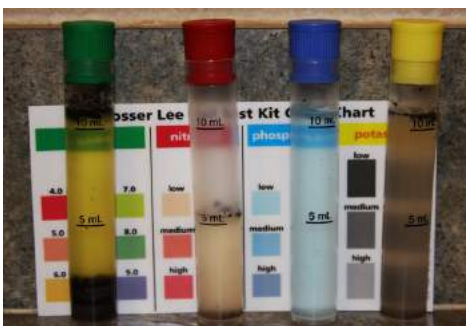
Figure 2-6. A soil test kit can help you determine the levels of phosphorus, nitrogen, potassium and pH of the soil on your property.
