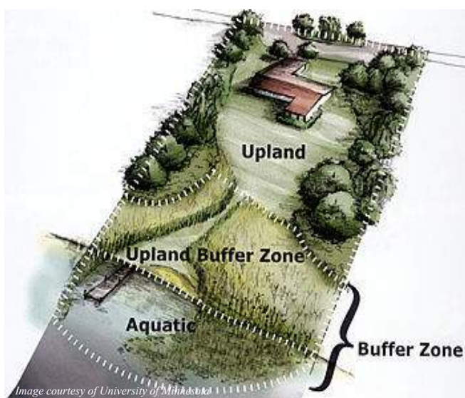
Figure 1-12. A vegetative buffer between water and upland land use protects water quality.
