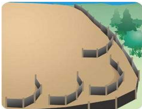
Figure 6-18. Ends turned up into “smiley face,” and room is left in front of fence to remove sediment.
