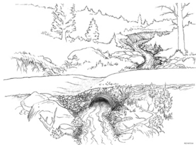
Figure 7-24. This sketch shows an armored overflow dip designed to reduce loss of road fill in the event of culvert failure.
